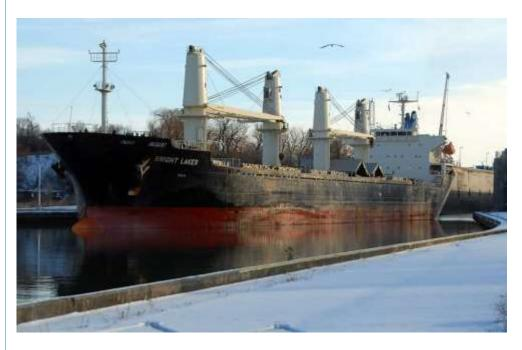
Ocean freighter transiting St. Lawrence Seaway: 1 inch reduction in water level means 100 tons less cargo.
