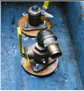
A good seacock installation, however note the use of stainless steel screws and nuts. Ideally these should be bronze and trimmed so as not to pose a danger to persons moving about the bilge.
