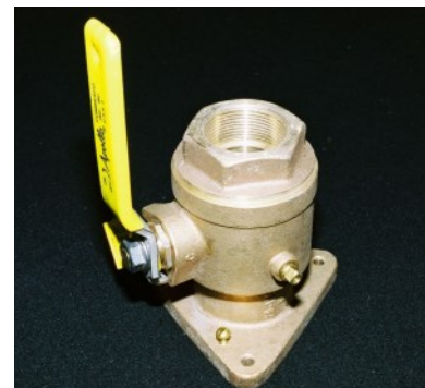
A bronze seacock. Note the screw on the mounting flange for connection of the bonding wire.
