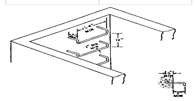
FIGURE D-1.—Suggested design for rungs on individual-rung ladders.
