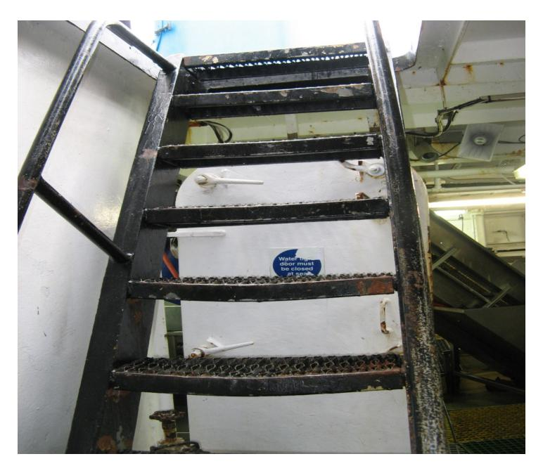
29 CFR 1910.27(b)(1)(v): "The rungs of an individual-rung ladder shall be so designed that the foot cannot slide off the end."
