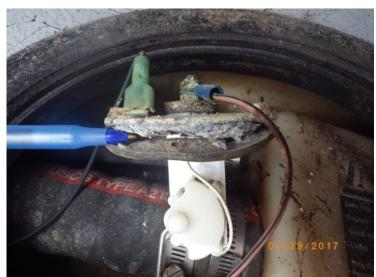
Close up of the corrosion on the sending unit. This expansion of material forced open the seal between the sending unit and the tank.
