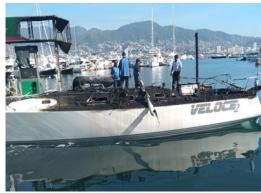
Unfortunately, we see these types of accidents quite often, due to the lack of responsibility of the boat operator in double checking the proper ventilation of the engine and not following the basic safety steps to refuel.
