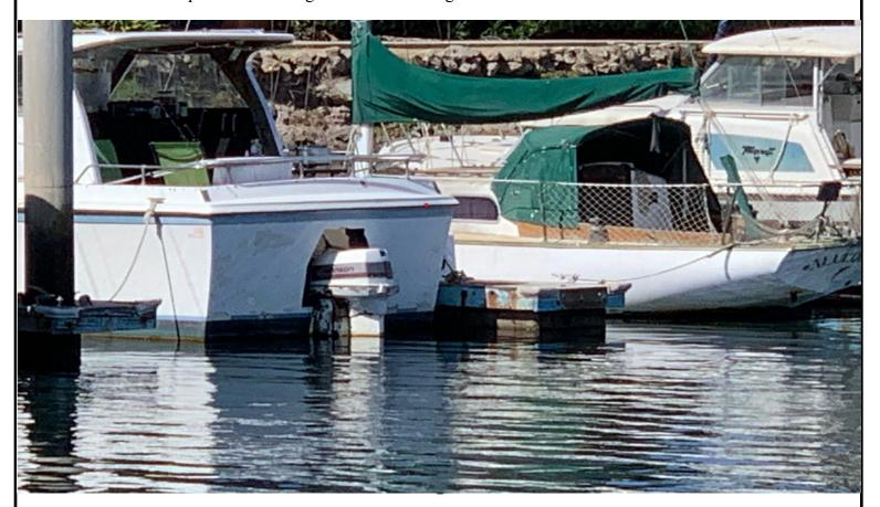
Note the professionally cut out transom, adequate mount above the waterline, bondo filled old exhaust exits, self flooding aft cockpit with period correct two stroke Johnson.
