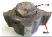
Figure 2: Accommodation ladder connection pin with severe corrosion over the pin's fracture surface & sidewall and on the surface of the hub.
