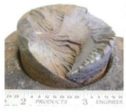
Figure 3: Surface corrosion and contamination are evident on the fracture surface of the failed turntable pin. Severe corrosion pits and surface cracks are also visible on the sidewall, which could have provided an indicator of the pin's unsafe condition prior to failure.
