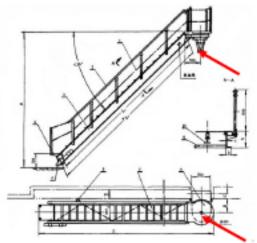
Figure 1: Pin location on the Accommodation Ladder Turntable
