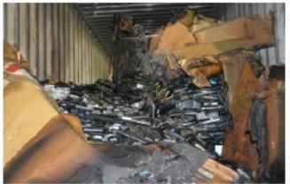
Burnt lithium batteries in fiberboard boxes.
