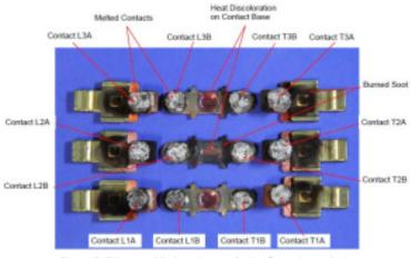
Figure 3: Disassembled contactor during forensic analysis (Image courtesy Chevron North America)
