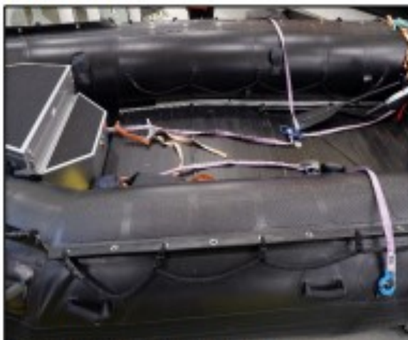
Figure 1 -Zodiac after bladder failure. Deformation to the deck is visible.
