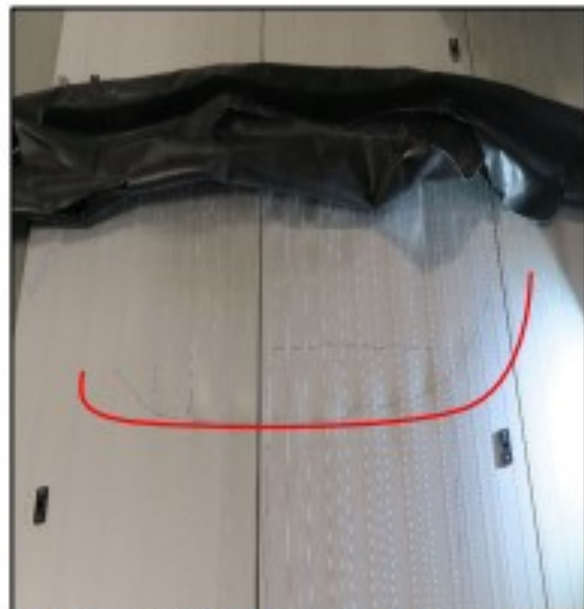
Figure 2 – Ruptured keel bladder and the view of the underside of the metal hull. The red line has been added to highlight the deformities in the hull metal due to the keel bladder rupture.
