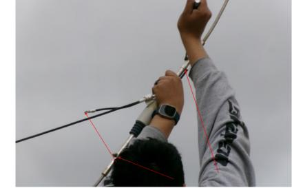
Jumper wire connected across the insulator removed from the clip here.
