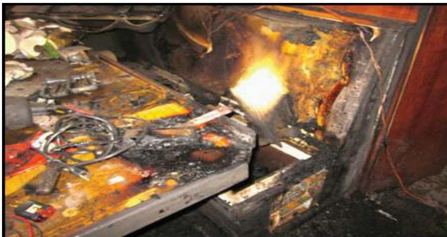
A nasty electrical heater fire in a bench seat, commercial fishing vessel.
