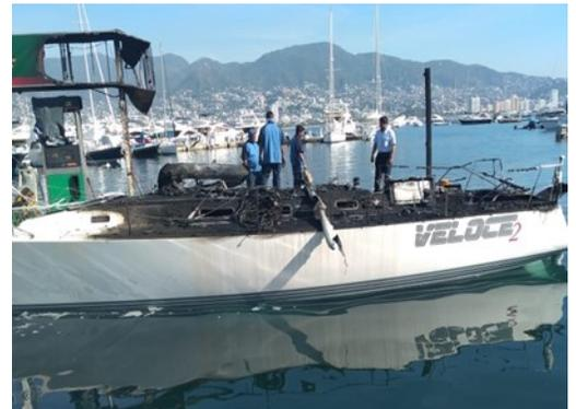
Unfortunately, we see these types of accidents quite often, due to the lack of responsibility of the boat operator in double checking the proper ventilation of the engine and not following the basic safety steps to refuel.
