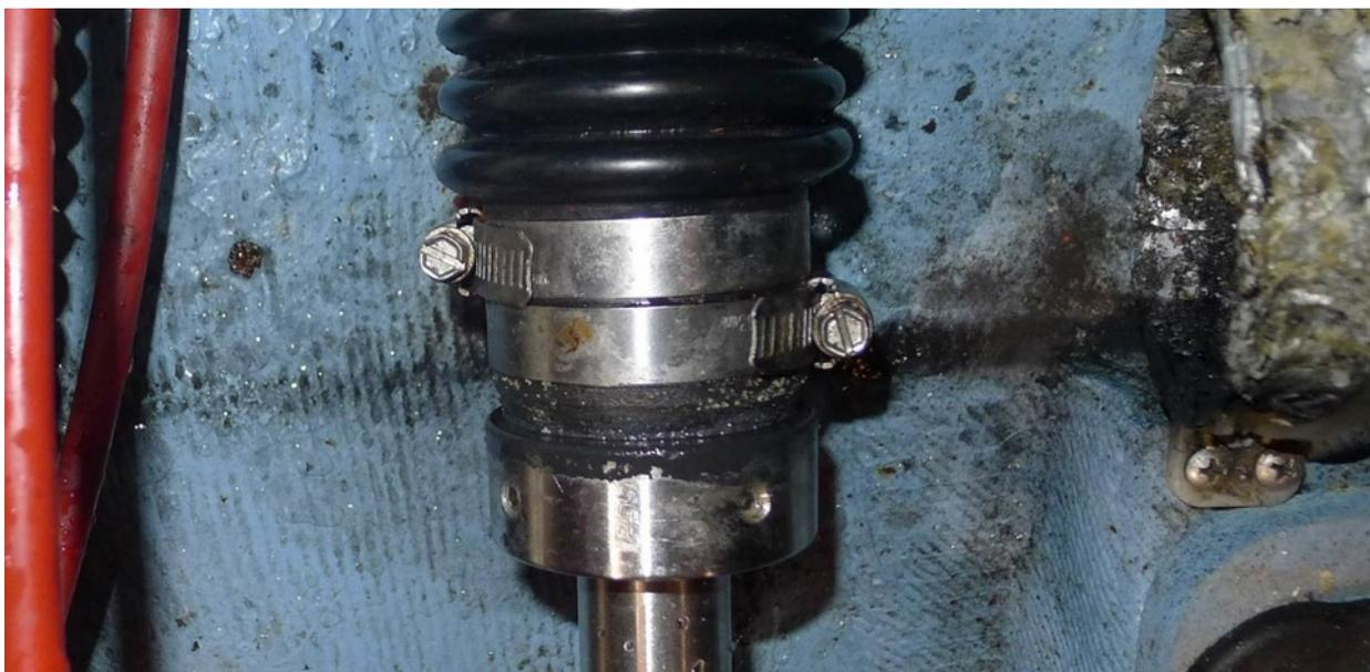
Note the black sling line on the hull from this shaft seal. This unit is worn and was slinging excessive water onto the fuel filter which was mounted just up to the left in the photo, causing corrosion on the fuel hose clamps and fittings.
