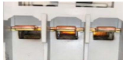
Figure 2: Welded contactors
