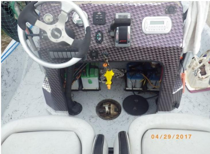
**Deck plate removed to gain access to the fuel sending unit.**
