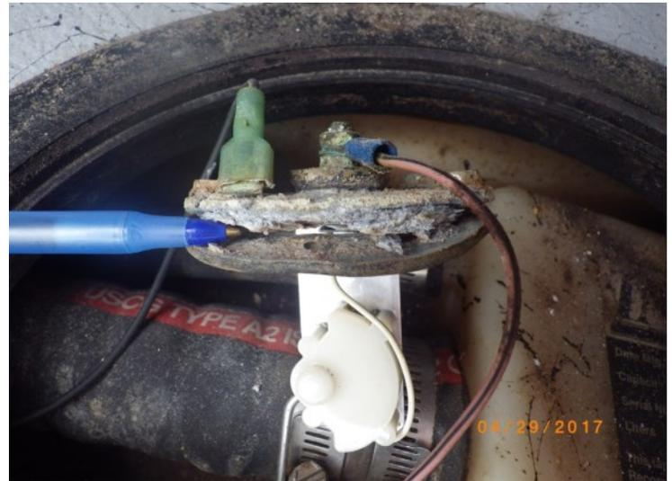
**Close up of the corrosion on the sending unit. This expansion of material forced open the seal between the sending unit and the tank.**
