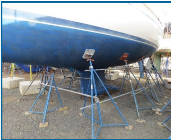
Marine jack stands connected with piping and clamps.
