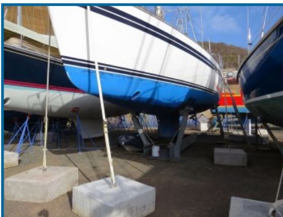
Yacht strapped to the ground using cargo straps, cement blocks.
