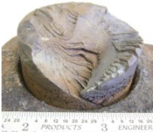
*Figure 3: Surface corrosion and contamination are evident on the fracture surface of the failed turntable pin. Severe corrosion pitting and surface cracks are also visible on the sidewall, which could have provided an indicator of the pin's unsafe condition prior to failure.*
