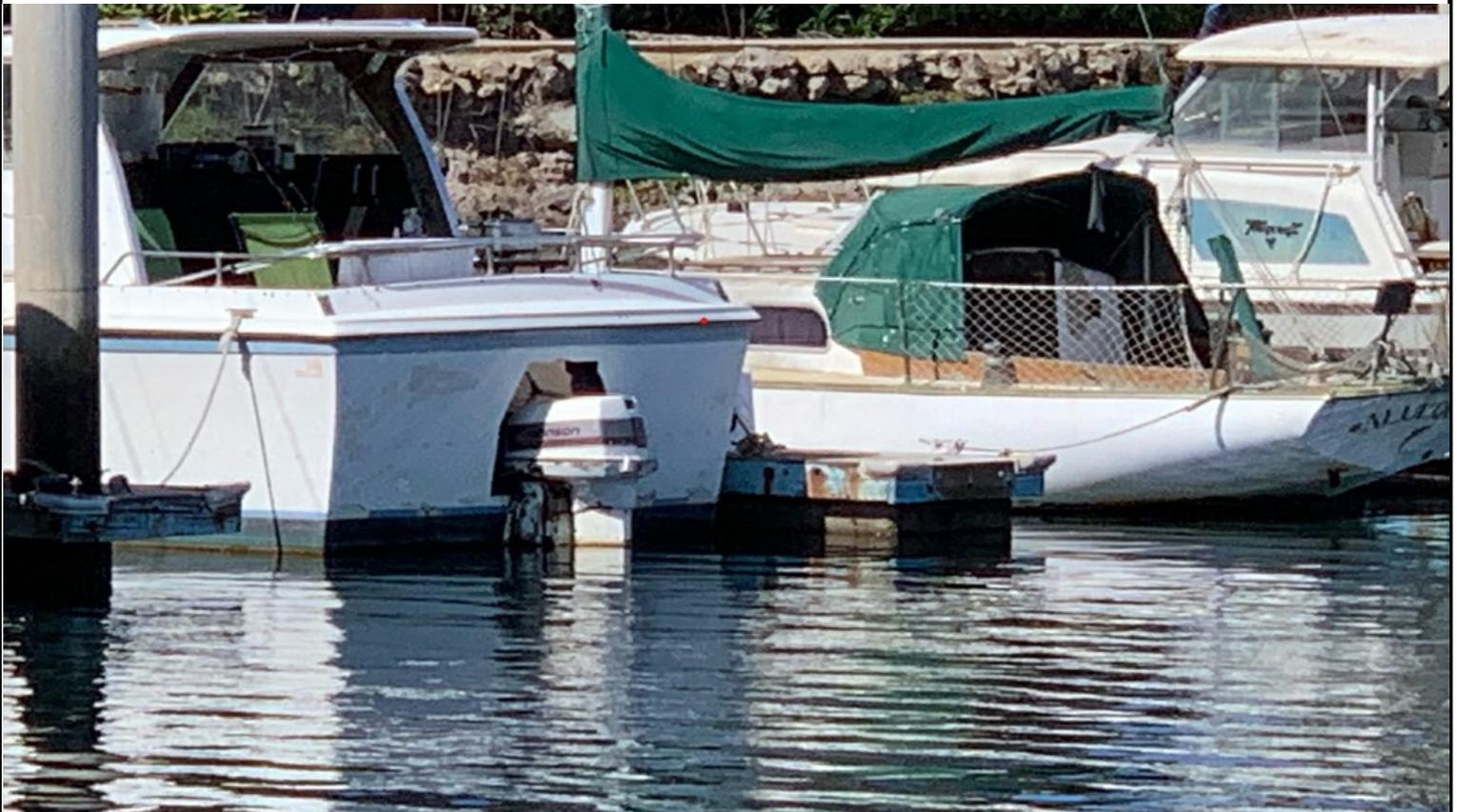
Note the professionally cut out transom, adequate mount above the waterline, bondo filled old exhaust exits, self flooding aft cockpit with period correct two stroke Johnson.
