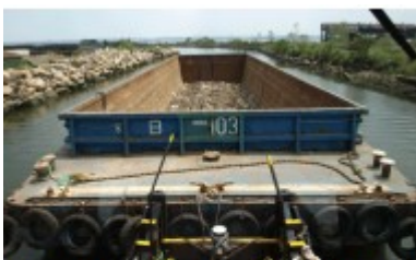
Pushing a light scrap barge out a narrow channel. With both knees against the barge, she pushes straight out.
