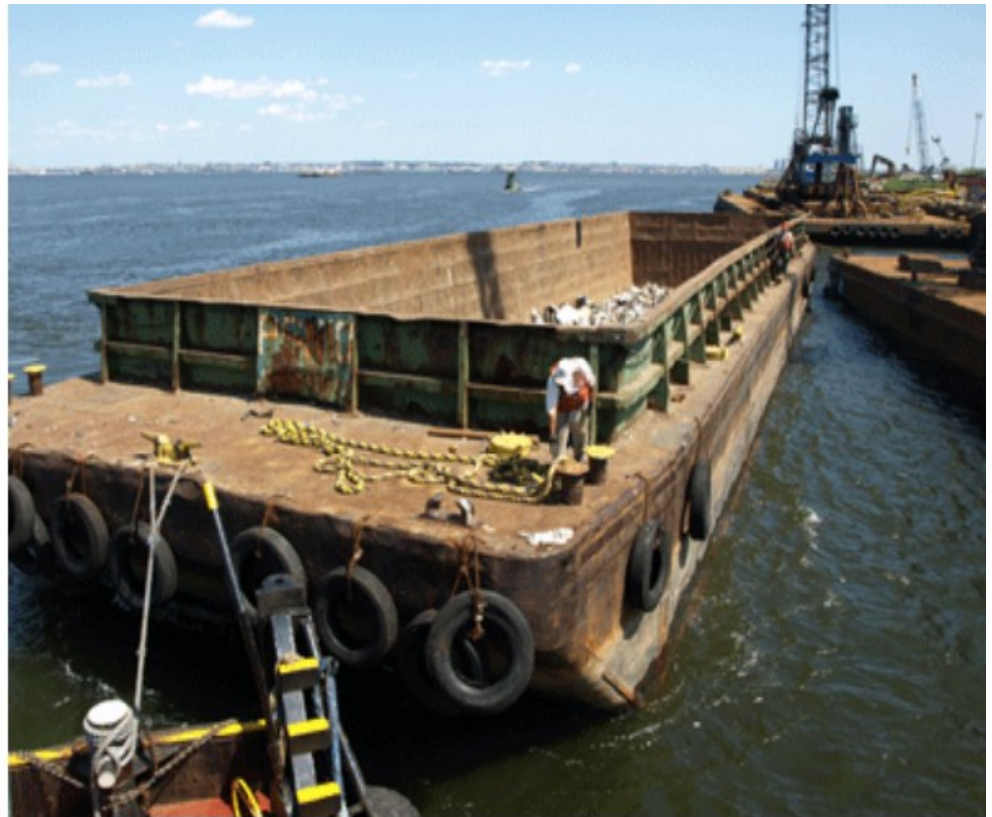
Backing a barge over to another barge – just keep the headline pointing in the way that you want the barge to go.
