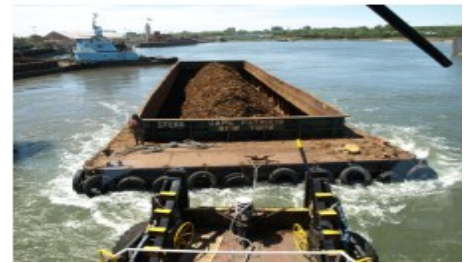
Backing a hopper loaded with 1,500 tons of shredded steel drawing 15 ft ¼ mile from the barge racks to shipside. This barge move takes 35 minutes on push wires but only 20 minutes on one line.
