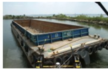
As we approach the first 90 degree turn to port, I shift the boat over to the port stern. This gives a little more leverage for pushing the stern to starboard and the bow to port and also keeps the tug's wheels in good water as it is shallow off to starboard.
