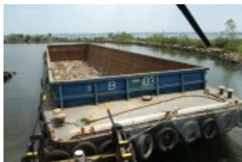
As we approach the first 90 degree turn to port, I shift the boat over to the port stern. This gives a little more leverage for pushing the stern to starboard and the bow to port and also keeps the tug's wheels in good water as it is shallow off to starboard.
